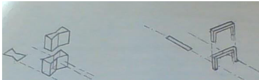
Fig 6: Interlocking of stones
